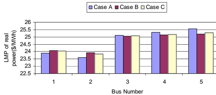
Figure 4. LMP of real power (\$/MWh) for low load under three Cases
