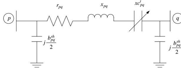
Figure 1. Pi-representation of transmission line with TCSC
