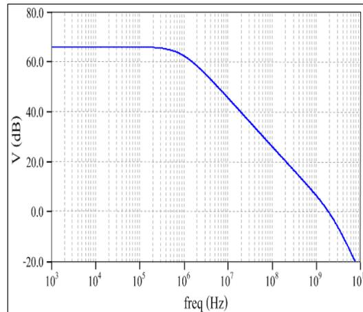
Figure 18. Gain curve for 180nm process nodes
