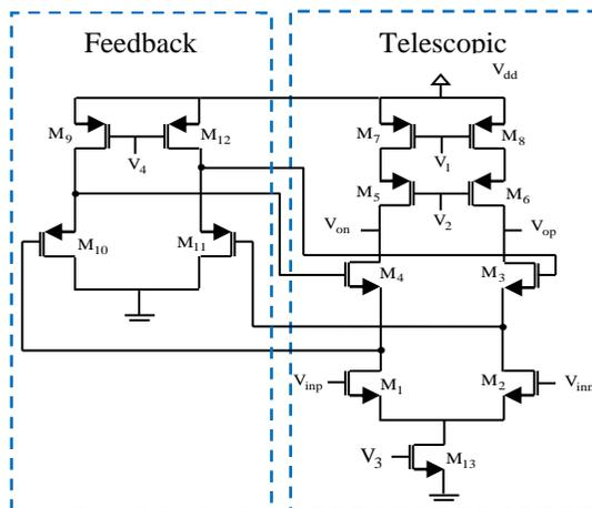
Figure 1. Schematic of the Regulated Telescopic OTA
