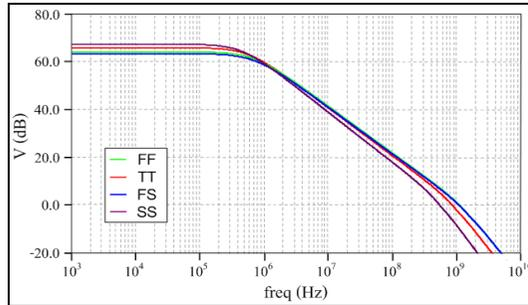
Figure 5. Process corners post-layout simulation for gain curve
