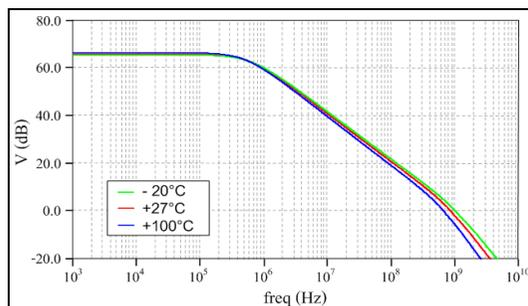
Figure 6. Gain curve with temperature variation from  $-20^{\circ}\text{C}$  to  $+100^{\circ}\text{C}$
