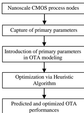
Figure 8. Synoptic of Nano CMOS OTA performance prediction
