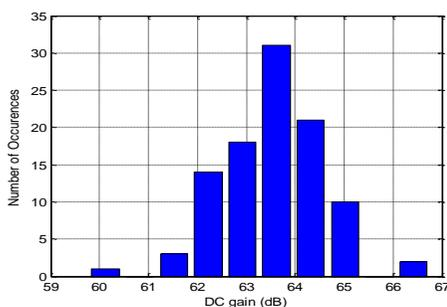
Figure 7. Histogram of 100-run Monte-Carlo simulation showing the effect of  $\pm 10\%$  process parameters mismatches on DC gain
