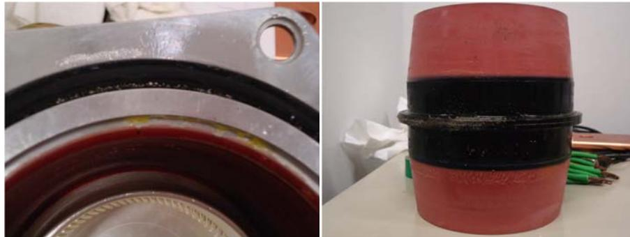
Figure 13 busbar socket with pollutants
