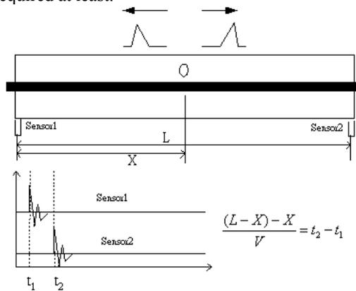
Figure 5. Diagram of time flying method
