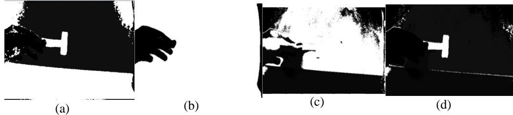
Figure 9. (a) Hue back projection image, (b) Saturation back projection image, (c) Value back projection image, (d) Combined of all back projection image
