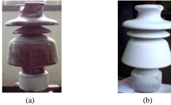
Figure 1. Pictures of non coated (a) and RTV coated (b) samples
