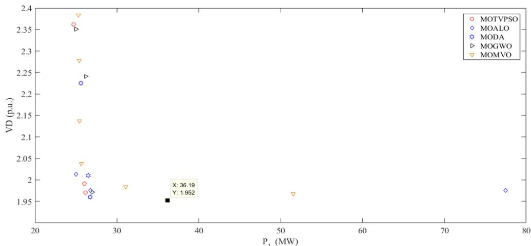
Figure 13. The best-obtained Pareto-fronts of MOTVPSO, MOALO, MODA, MOGWO, and MOMVO to minimize the total voltage deviation in the IEEE 57-bus.
