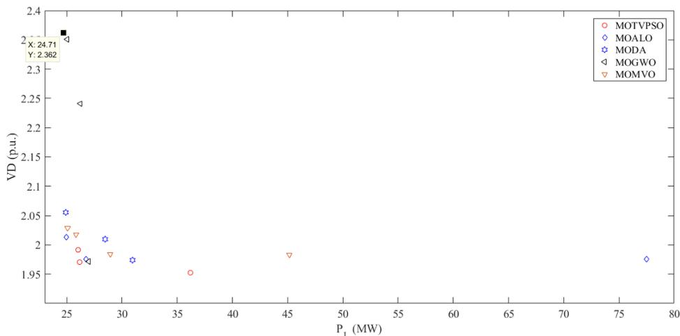
Figures 12. The best-obtained Pareto-fronts of MOTVPSO, MOALO, MODA, MOGWO, and MOMVO to minimize real power loss in the IEEE 57-bus.
