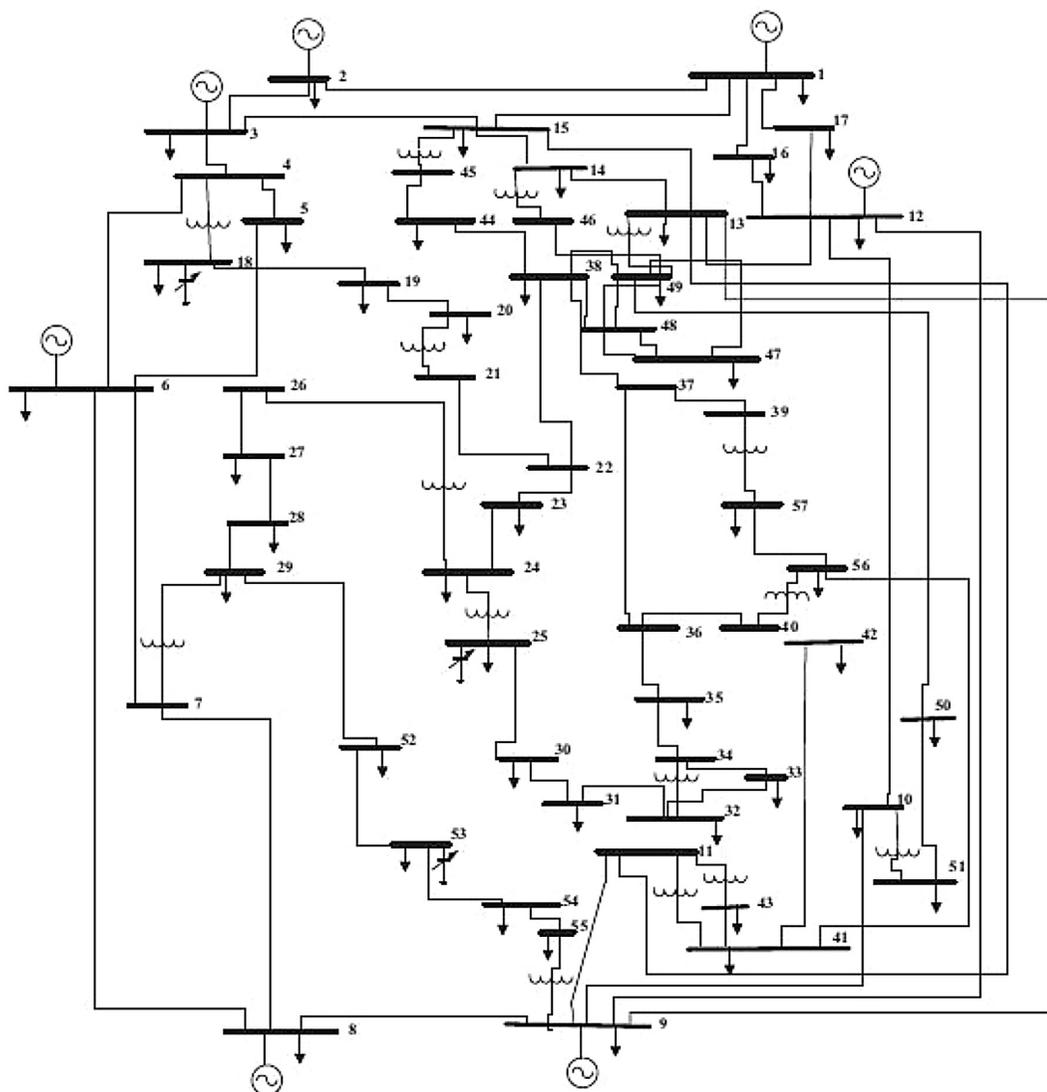
Figure 6. The single-line diagram of the IEEE 57-bus [37].
