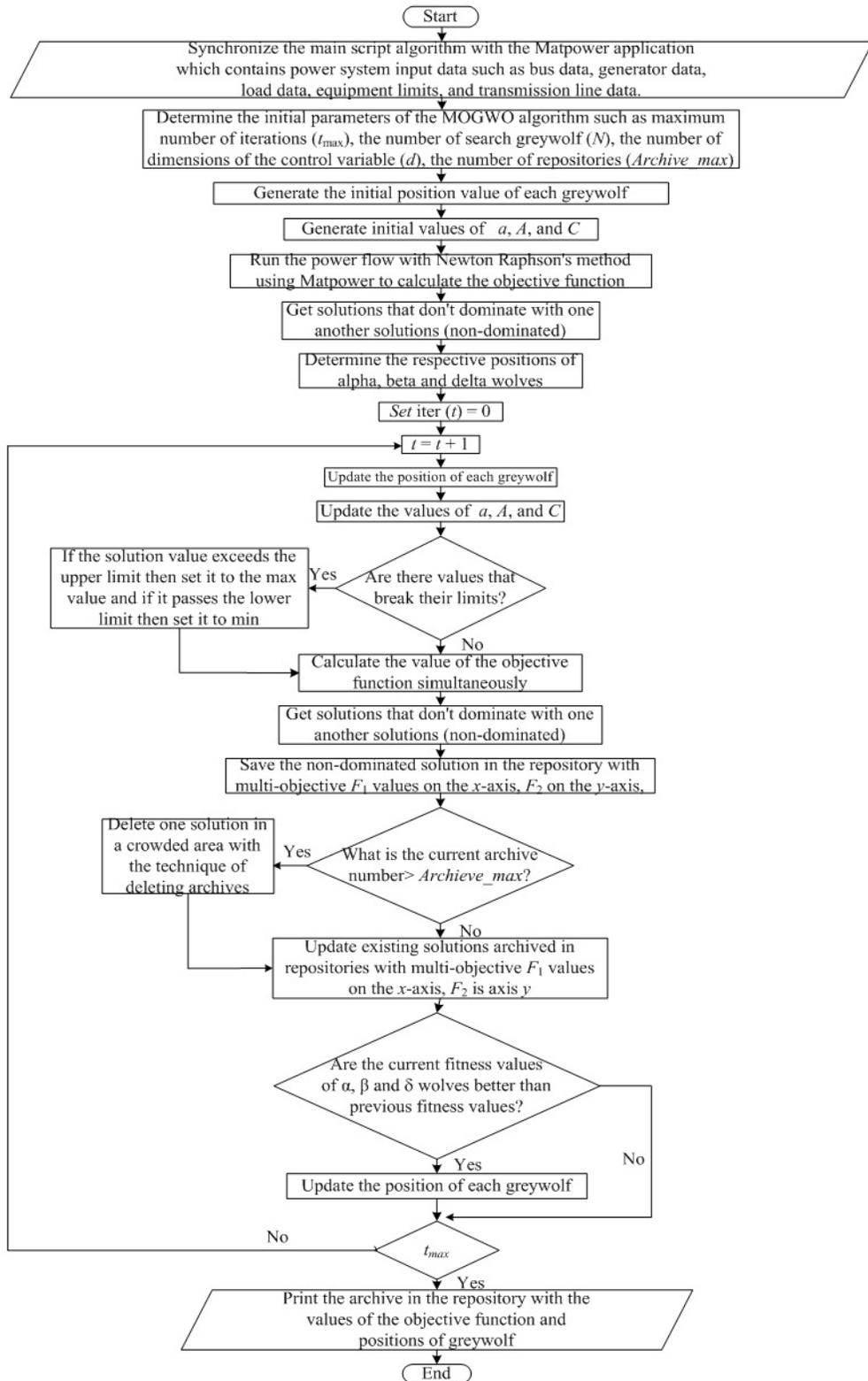
Figure 4. Flowchart of MOGWO algorithm
