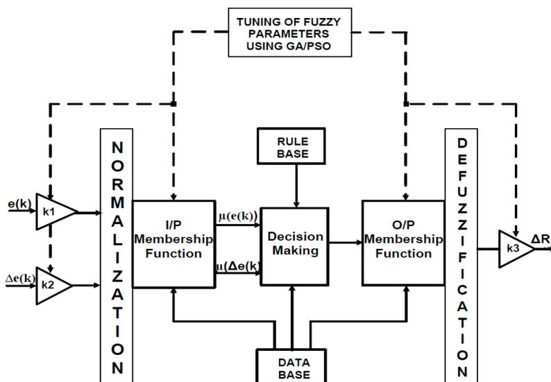
Figure 7. Block diagram of GA/PSO based fuzzy
