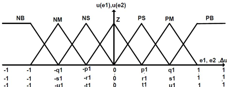
Figure 5. Input/output variable fuzzy membership function
