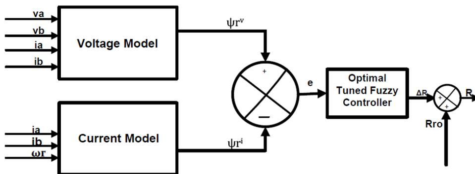
Figure 2. Proposed RF MRAC for rotor resistance estimation
