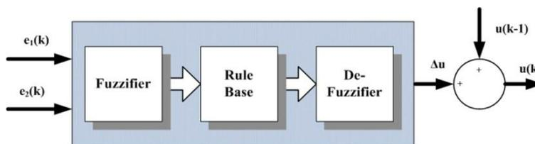
Figure 4. Block diagram of a fuzzy controller
