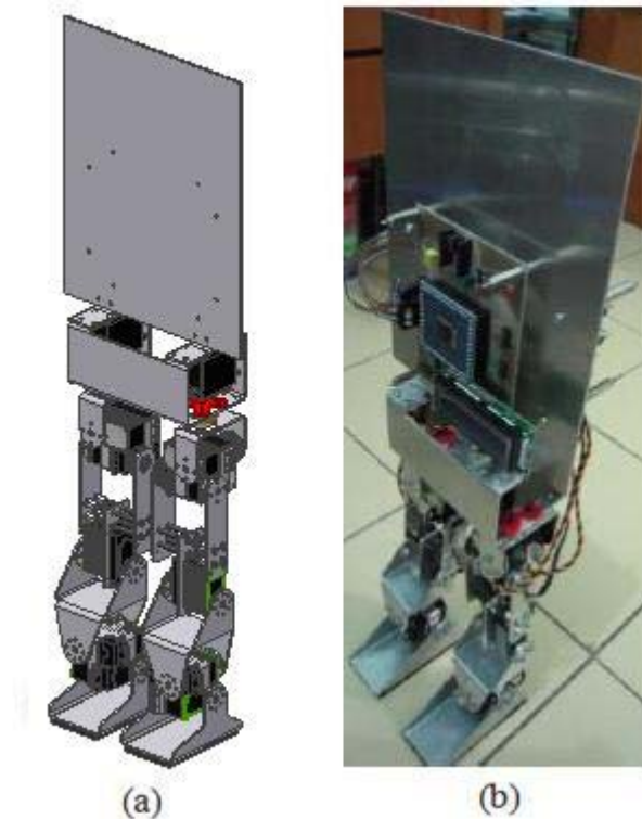
Figure 6. The manufactured design: (a) Mechanical design simulation; (b) Realization, along with electrical system.
