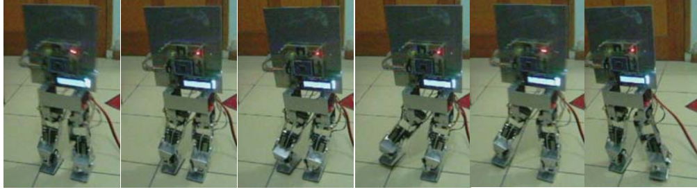
Figure 15. Image sequence extracted from video of ArtRo walking to the side (every sixth frame).
