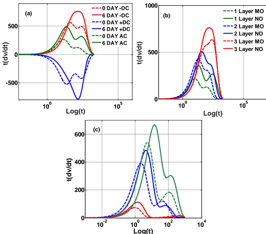
Figure 10. Variation  $t(dv/dt)$  curve of charge decay curve obtained under AC and DC voltage (a) AC and DC voltage profiles of virgin OIPs and thermally aged at 120 C, (b) layers for transformer OIPs and titania nanoparticles dispersed OIP materials of virgin material, and (c) with thermal aged material with three layers
