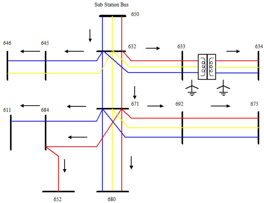
Figure 9. Modified IEEE 13-Bus unbalanced radial distribution network (URDN)
