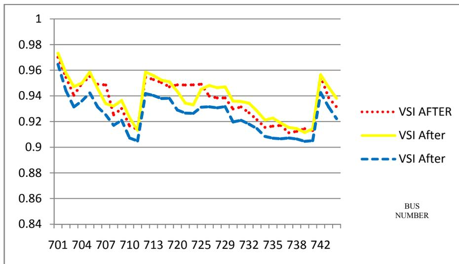
Figure 14. VSI of 3 phases after capacitor compensation in IEEE 37 bus test system
