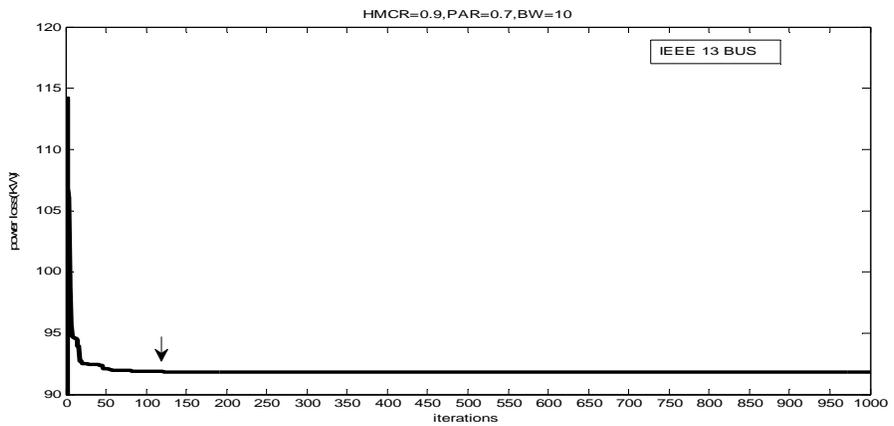
Figure 3. Effect of choosing high values of HSA parameters on convergence of IEEE 13 bus test system solution
