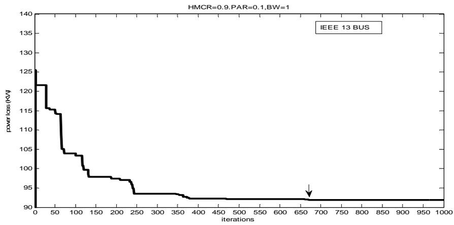
Figure 2. Effect of choosing low values of HSA parameters on convergence of IEEE 13 bus test system solution
