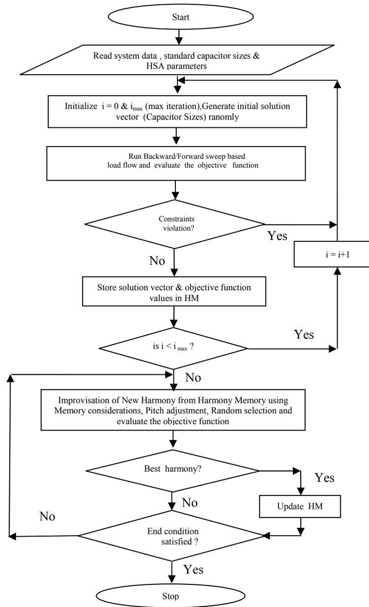
Figure 8. Flow chart of proposed HS algorithm
