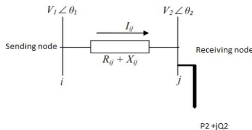
Figure 1. Branch of radial distribution network
