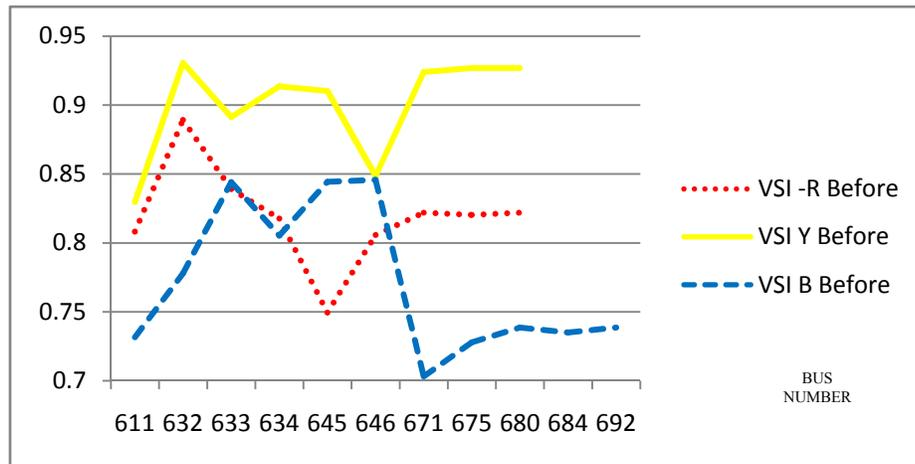
Figure 10. VSI of three phases before capacitor compensation in IEEE 13 bus test system
