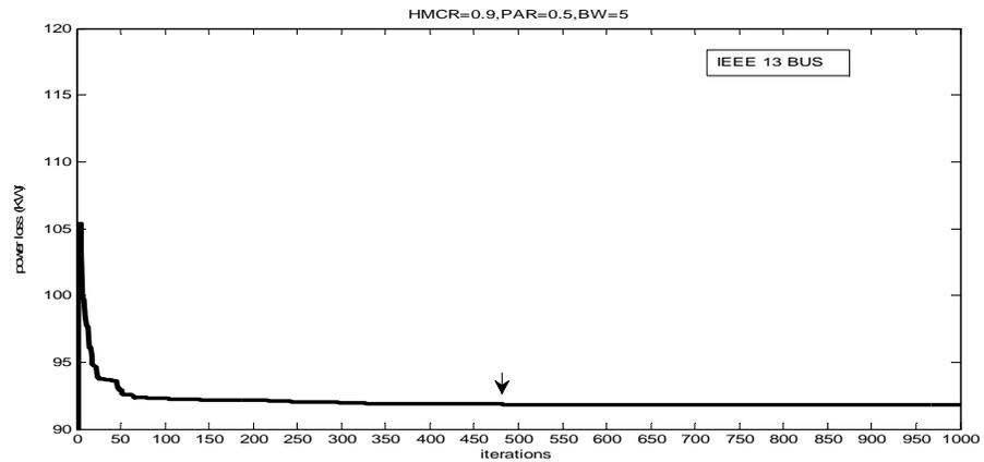
Figure 4. Effect of chosen values of HSA parameters on convergence of IEEE 13 bus test system solution
