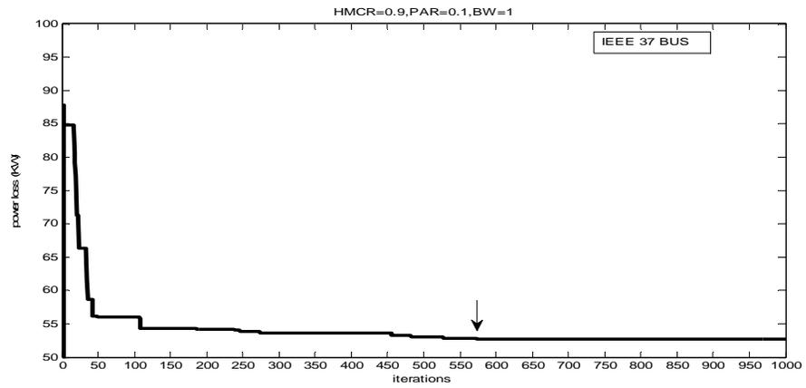
Figure 5. Effect of choosing low values of HSA parameters on convergence of IEEE 37 bus test system solution
