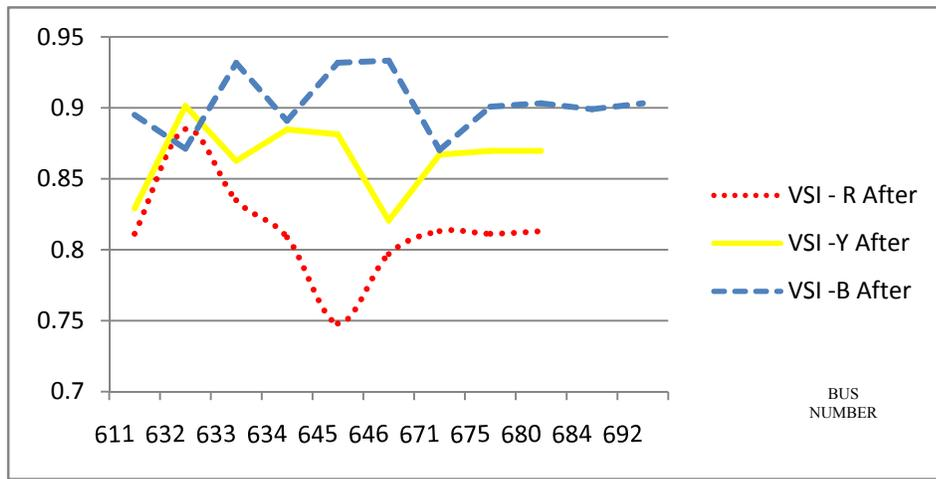
Figure 11. VSI of three phases after capacitor compensation in IEEE 13 bus test system
