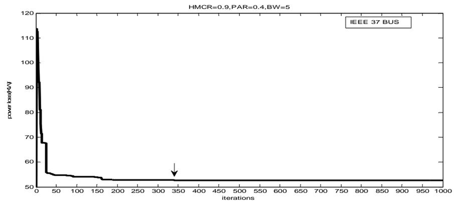
Figure 7. Effect of chosen values of HSA parameters on convergence of IEEE 37 bus test system solution
