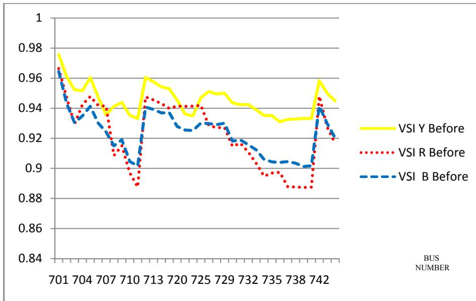
Figure 13. VSI of 3 phases before capacitor compensation IEEE 37 bus test system
