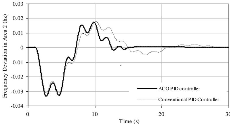
Figure 16. Controlled response with GRC non-linearity unit (delf2)
