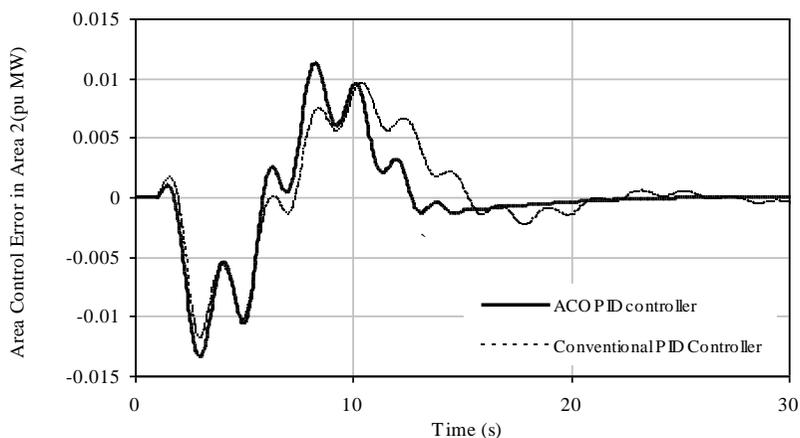
Figure 22. Controlled response with GRC non-linearity unit (ACE2)
