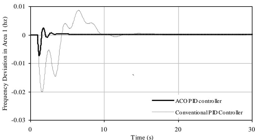
Figure 6. Controlled response without GRC non-linearity unit ( $\delta F1$ )
