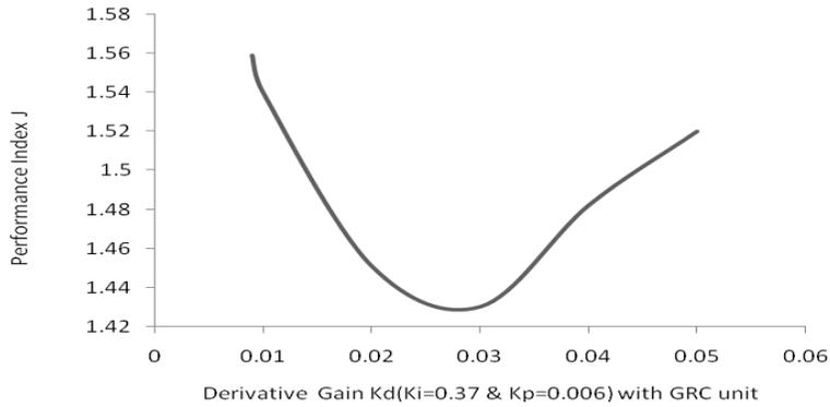
Figure 4. Cost function vs  $K_d$  considering GRC
