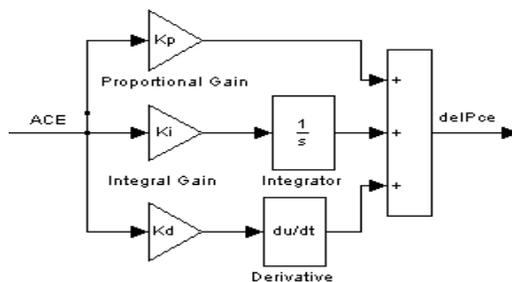
Figure 2. Structure of PID controller
