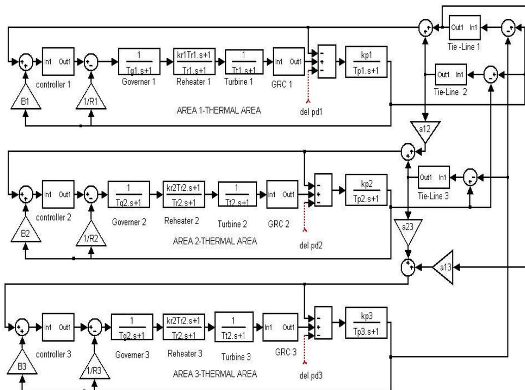
Figure 1. Transfer function model of three area interconnected thermal power systems with GRC Non-linearity
