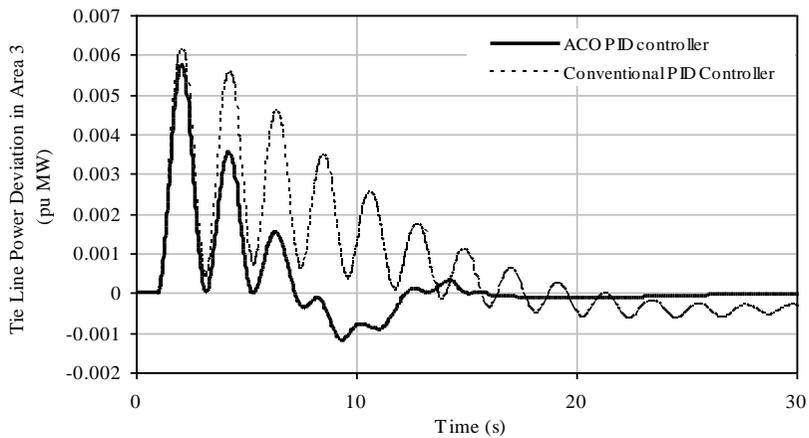
Figure 20. Controlled response with GRC non-linearity unit (delPtie3)
