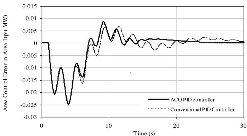
Figure 21. Controlled response with GRC non-linearity unit (ACE1)
