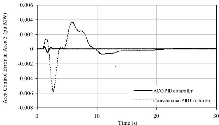
Figure 14. Controlled response without GRC non-linearity unit (ACE3)
