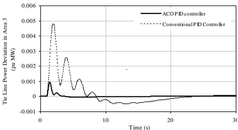
Figure 11. Controlled response without GRC non-linearity unit (delPtie3)
