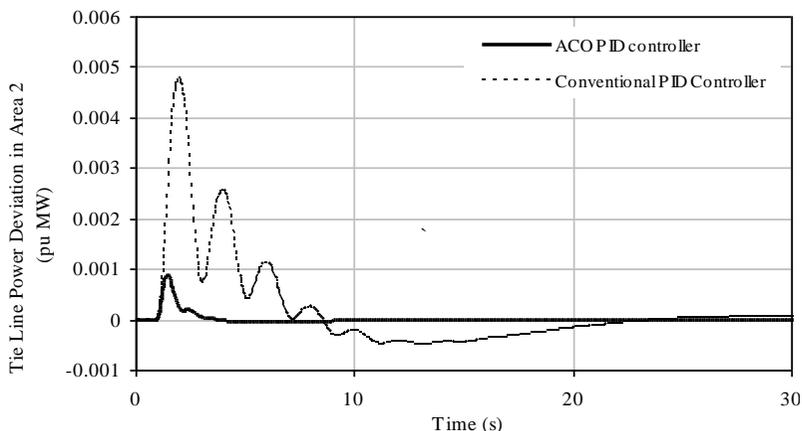
Figure 10. Controlled response without GRC non-linearity unit (delPtie2)
