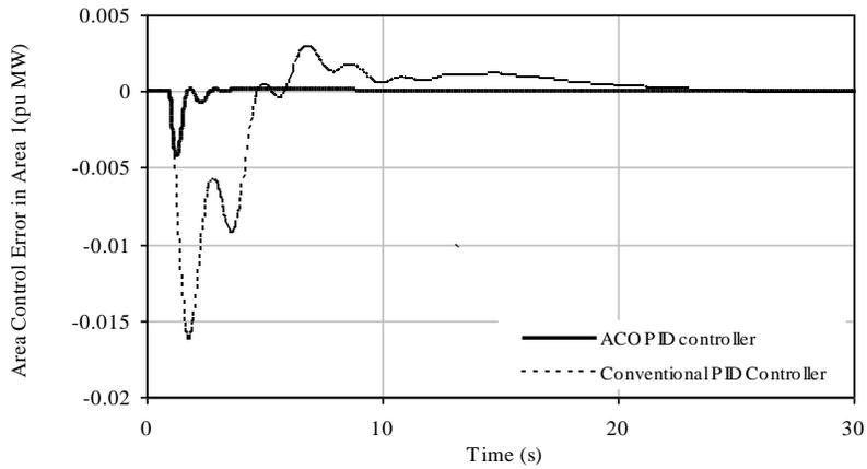
Figure 12. Controlled response without GRC non-linearity unit (ACE1)
