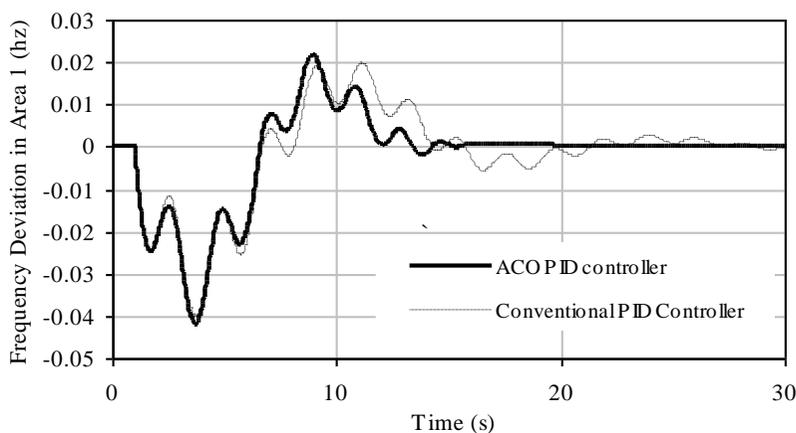
Figure 15. Controlled response with GRC non-linearity unit (delF1)
