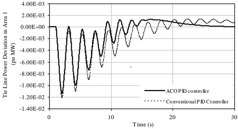
Figure 18. Controlled response with GRC non-linearity unit (delPtie1)
