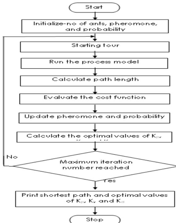
Figure 5. Flow chart of ACO technique
