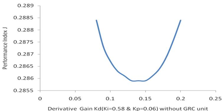
Figure 3. Cost function vs  $K_d$  without GRC
