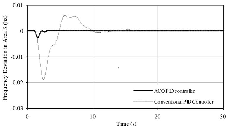
Figure 8. Controlled response without GRC non-linearity unit ( $\Delta f_3$ )
