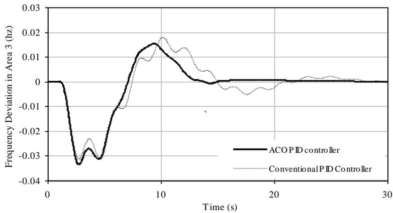
Figure 17. Controlled response with GRC non-linearity unit (delf3)
