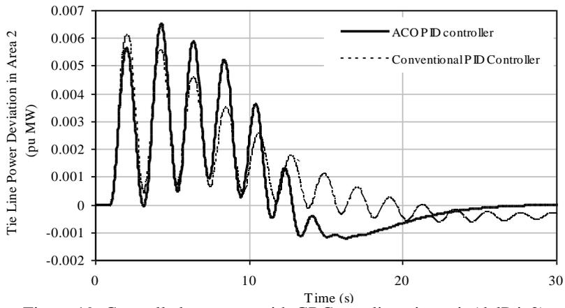
Figure 19. Controlled response with GRC non-linearity unit (delPtie2)
