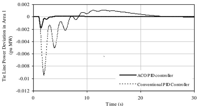
Figure 9. Controlled response without GRC non-linearity unit ( $\Delta P_{tie1}$ )
