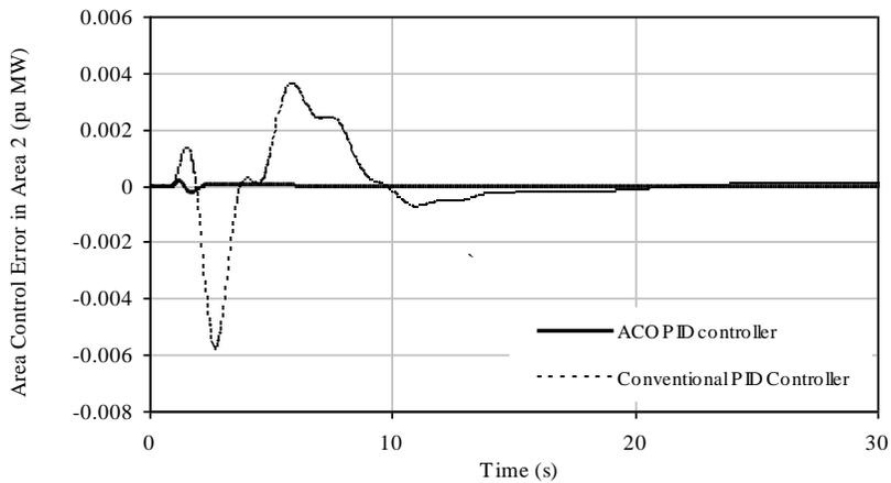
Figure 13. Controlled response without GRC non-linearity unit (ACE2)
