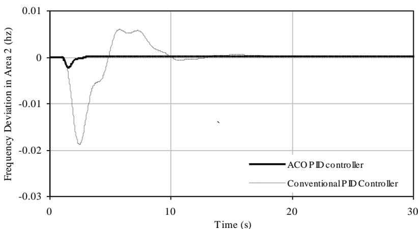
Figure 7. Controlled response without GRC non-linearity unit ( $\delta F2$ )
